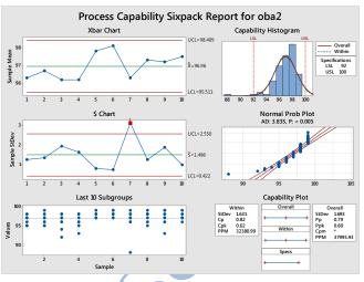
Figure 5: X-bar Chart, S-Chart plots and Capability Plot for Oba2
