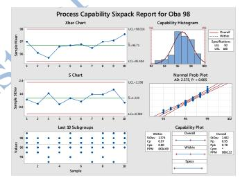
Figure 4: X-bar Chart, S-Chart plots and Capability Plot for Oba98
